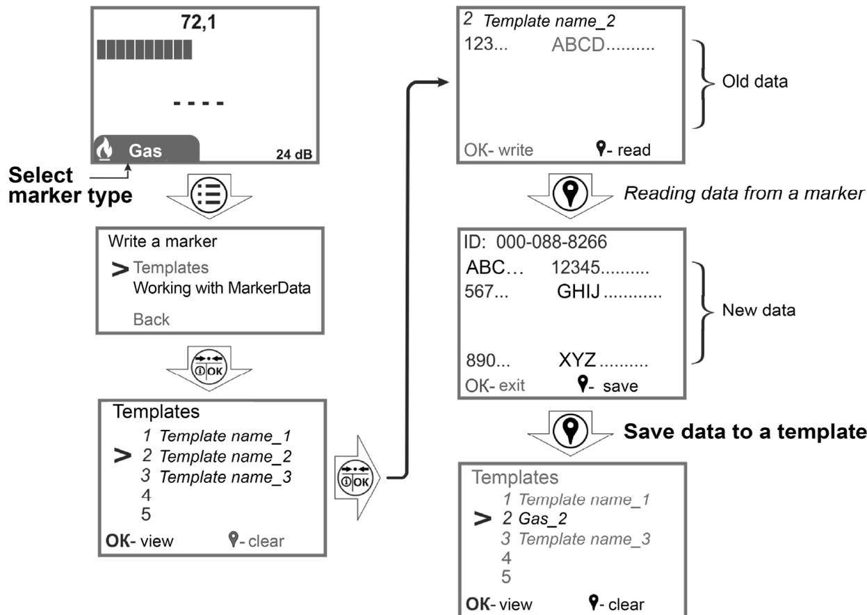
Figure 4.2.4 – Reading data from a marker into a template
