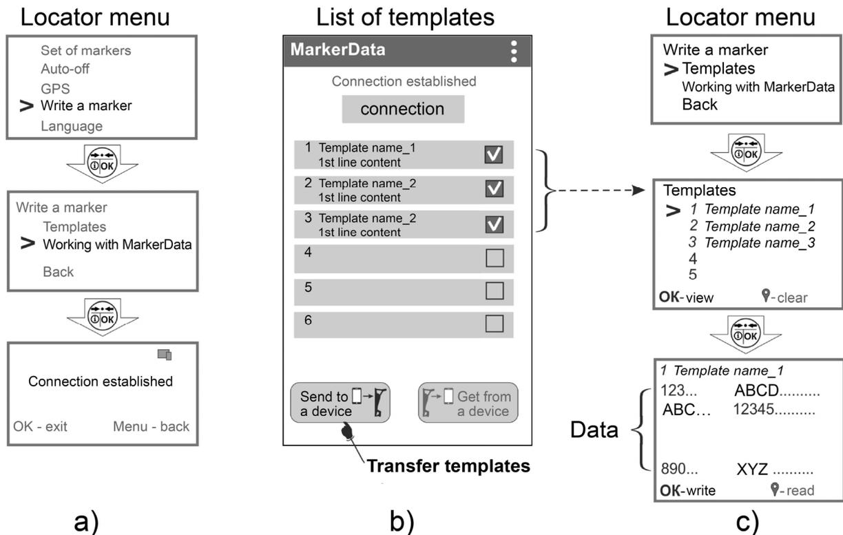
Figure 4.2.2 – Transferring templates
