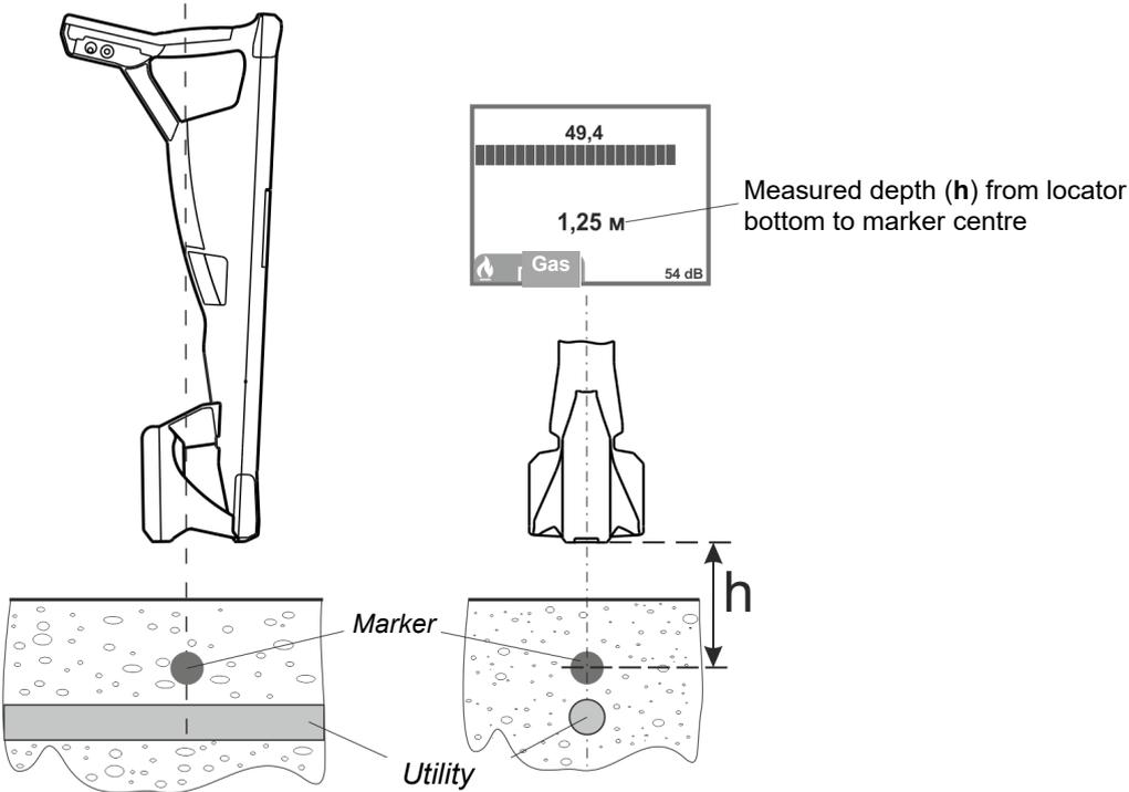
Figure 3.2c – Depth measurement
